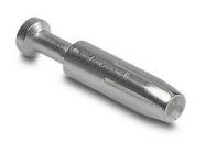
ZIPport crimp contact, female, 16 amp, accepts wire size 20 AWG, silver-plated copper alloy. Package of 100. For use with ZIPport multi-wire female inserts rated for 16 amps.
