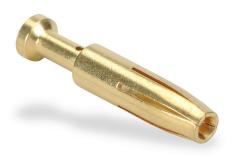
ZIPport crimp contact, female, 16 amp, accepts wire size 20 AWG, gold-plated copper alloy. Package of 100. For use with ZIPport multi-wire female inserts rated for 16 amps.
