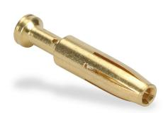
ZIPport crimp contact, female, 16 amp, accepts wire size 18 AWG, gold-plated copper alloy. Package of 100. For use with ZIPport multi-wire female inserts rated for 16 amps.
