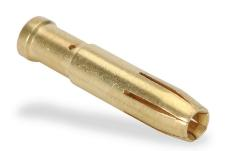
ZIPport crimp contact, female, 16 amp, accepts wire size 12 AWG, gold-plated copper alloy. Package of 100. For use with ZIPport multi-wire female inserts rated for 16 amps.
