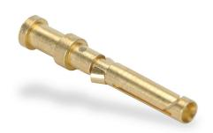
ZIPport crimp contact, female, 10 amp, accepts wire size 26-22 AWG, gold-plated copper alloy. Package of 100. For use with ZIPport multi-wire female inserts rated for 10 amps.
