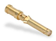
ZIPport crimp contact, female, 10 amp, accepts wire size 16 AWG, gold-plated copper alloy. Package of 100. For use with ZIPport multi-wire female inserts rated for 10 amps.
