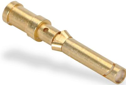
ZIPport crimp contact, female, 10 amp, accepts wire size 16 AWG, gold-plated copper alloy. Package of 100. For use with ZIPport multi-wire female inserts rated for 10 amps.
