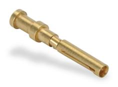
ZIPport crimp contact, female, 10 amp, accepts wire size 14 AWG, gold-plated copper alloy. Package of 100. For use with ZIPport multi-wire female inserts rated for 10 amps.
