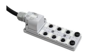
ZIPport junction block, 8 ports, 5-pin M12 sockets, 5-wire, 48 VDC, 3A, power and PNP LED indicator(s), 5m integrated cable, IP67. (2) port caps for unused ports included.
