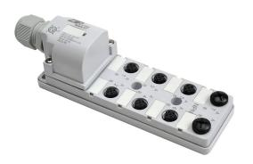
ZIPport junction block, 8 ports, 5-pin M12 sockets, 5-wire, 48 VDC, 3A, power and NPN LED indicator(s), field-wired connection, IP67. (2) port caps for unused ports included.
