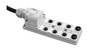
ZIPport junction block, 8 ports, 5-pin M12 sockets, 5-wire, 48 VDC, 3A, power and NPN LED indicator(s), 5m integrated cable, IP67. (2) port caps for unused ports included.
