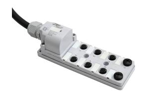
ZIPport junction block, 8 ports, 5-pin M12 sockets, 5-wire, 150 VAC/VDC, 3A, 5m integrated cable, IP67. (2) port caps for unused ports included.
