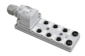
ZIPport junction block, 8 ports, 5-pin M12 sockets, 4-wire, 48 VDC, 3A, power and PNP LED indicator(s), field-wired connection, IP67. (2) port caps for unused ports included.
