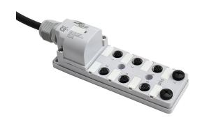
ZIPport junction block, 8 ports, 5-pin M12 sockets, 4-wire, 48 VDC, 3A, power and PNP LED indicator(s), 5m integrated cable, IP67. (2) port caps for unused ports included.
