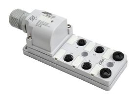
ZIPport junction block, 6 ports, 5-pin M12 sockets, 4-wire, 48 VDC, 3A, power and PNP LED indicator(s), field-wired connection, IP67. (2) port caps for unused ports included.
