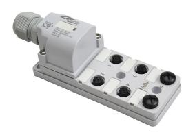
ZIPport junction block, 6 ports, 5-pin M12 sockets, 4-wire, 48 VDC, 3A, power and NPN LED indicator(s), field-wired connection, IP67. (2) port caps for unused ports included.
