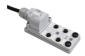
ZIPport junction block, 6 ports, 5-pin M12 sockets, 4-wire, 48 VDC, 3A, power and NPN LED indicator(s), 5m integrated cable, IP67. (2) port caps for unused ports included.
