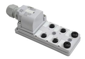
ZIPport junction block, 6 ports, 5-pin M12 sockets, 4-wire, 150 VAC/VDC, 3A, field-wired connection, IP67. (2) port caps for unused ports included.
