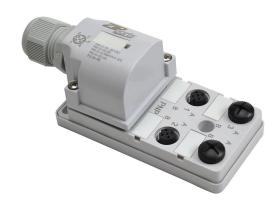
ZIPport junction block, 4 ports, 5-pin M12 sockets, 5-wire, 48 VDC, 3A, power and PNP LED indicator(s), field-wired connection, IP67. (2) port caps for unused ports included.
