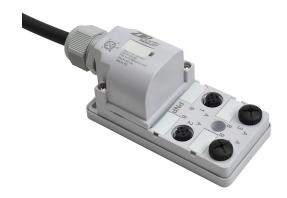
ZIPport junction block, 4 ports, 5-pin M12 sockets, 5-wire, 48 VDC, 3A, power and PNP LED indicator(s), 5m integrated cable, IP67. (2) port caps for unused ports included.
