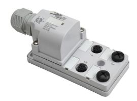
ZIPport junction block, 4 ports, 5-pin M12 sockets, 5-wire, 150 VAC/VDC, 3A, field-wired connection, IP67. (2) port caps for unused ports included.
