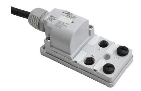
ZIPport junction block, 4 ports, 5-pin M12 sockets, 5-wire, 150 VAC/VDC, 3A, 5m integrated cable, IP67. (2) port caps for unused ports included.
