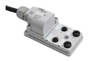
ZIPport junction block, 4 ports, 5-pin M12 sockets, 5-wire, 150 VAC/VDC, 3A, 5m integrated cable, IP67. (2) port caps for unused ports included.
