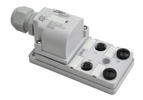
ZIPport junction block, 4 ports, 5-pin M12 sockets, 4-wire, 48 VDC, 3A, power and PNP LED indicator(s), field-wired connection, IP67. (2) port caps for unused ports included.
