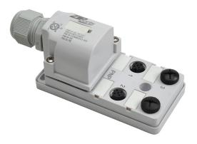
ZIPport junction block, 4 ports, 5-pin M12 sockets, 4-wire, 48 VDC, 3A, power and PNP LED indicator(s), field-wired connection, IP67. (2) port caps for unused ports included.
