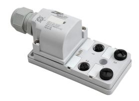
ZIPport junction block, 4 ports, 5-pin M12 sockets, 4-wire, 48 VDC, 3A, power and NPN LED indicator(s), field-wired connection, IP67. (2) port caps for unused ports included.
