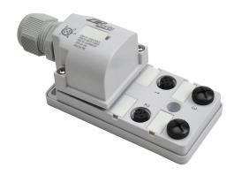
ZIPport junction block, 4 ports, 5-pin M12 sockets, 4-wire, 150 VAC/VDC, 3A, field-wired connection, IP67. (2) port caps for unused ports included.
