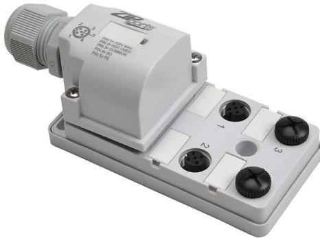
ZPport junction block, 4 ports, 5-pin M12 sockets, 4-wire, 150 VAC/VDC, 3A, field-wired connection, IP67. (2) port caps for unused ports included.
