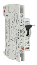
Eaton alarm/auxiliary contact, (2) SPDT contact(s), 2A @ 230VAC/0.5A @ 110VAC/VDC. For use with Eaton FAZ-NA series miniature circuit breakers.
