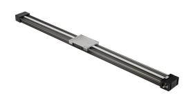
igus drylin series linear actuator assembly, W1080 twin rail, 90mm wide, 1000mm travel, toothed belt, 70mm pitch, hard-anodized aluminum rail.
