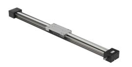
igus drylin series linear actuator assembly, W1040 twin rail, 74mm wide, 600mm travel, toothed belt, 70mm pitch, hard-anodized aluminum rail.
