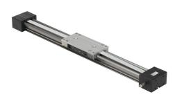
igus drylin series linear actuator assembly, W1040 twin rail, 74mm wide, 400mm travel, toothed belt, 70mm pitch, hard-anodized aluminum rail.
