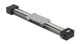
igus drylin series linear actuator assembly, W1040 twin rail, 74mm wide, 300mm travel, toothed belt, 70mm pitch, hard-anodized aluminum rail.
