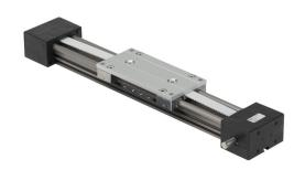
igus drylin series linear actuator assembly, W1040 twin rail, 74mm wide, 200mm travel, toothed belt, 70mm pitch, hard-anodized aluminum rail.
