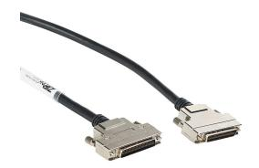
ZIPLink servo cable, 50-pin connector to 50-pin connector, shielded, twisted pair, 6.5ft/2m cable length. For use with SureServo amplifiers.
