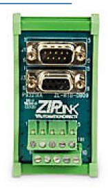
ZIPLink feedthrough communication module, 10-position terminal block to 9-pin D-sub male/female, DIN rail mount.
