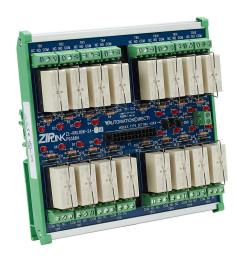
ZIPLink reduced-width relay output module, 16-point, sourcing, (16) Form C (SPDT) relays, LED indication, 24 VDC (coil), 8A at 250 VAC, 10A at 30 VDC, DIN rail mount. For replacement relays, use ZL-RELAY-24X4.
