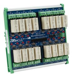
ZIPLink reduced-width relay output module, 16-point, sinking, (16) Form C (SPDT) relays, LED indication, 24 VDC (coil), 8A at 250 VAC, 10A at 30 VDC, DIN rail mount. For replacement relays, use ZL-RELAY-24X4.
