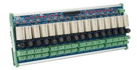
ZIPLink fused relay output module, 16-point, sourcing, (16) Form C (SPDT) relays, LED indication, 24 VDC (coil), 8A at 250 VAC, 8A at 30 VDC, DIN rail mount. For replacement relays, use ZL-RELAY-F24X4. Fuses sold separately.
