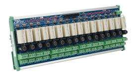
ZIPLink fused relay output module, 16-point, sinking, (16) Form C (SPDT) relays, LED indication, 24 VDC (coil), 8A at 250 VAC, 8A at 30 VDC, DIN rail mount. For replacement relays, use ZL-RELAY-F24X4. Fuses sold separately.
