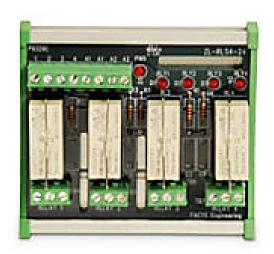
ZIPLink stand-alone relay output module, 4-point, (4) Form C (SPDT) relays, LED indication, 24 VDC (coil), 8A at 250 VAC, 10A at 30 VDC, DIN rail mount. For replacement relays, use ZL-RELAY-24X4.
