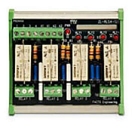
ZIPLink stand-alone relay output module, 4-point, (4) Form C (SPDT) relays, LED indication, 120 VAC (coil), 8A at 250 VAC, 10A at 30 VDC, DIN rail mount. For replacement relays, use ZL-RELAY-120X4.
