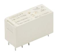
ZIPLink relay, replacement, 120 VAC (coil), 8A at 250 VAC, 10A at 30 VDC. Package of 4. For use with ZL-RLS1-120 and ZL-RLS4-120 relay modules.
