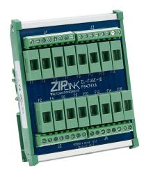
ZIPLink reduced-width stand-alone fuse module, 16-point, user-supplied external fuse, 250 VAC/VDC, 5A/circuit, DIN rail mount.
