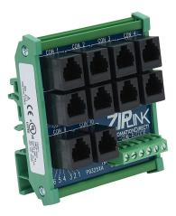
ZIPLink port distribution communication module, 10 ports, RJ12 6P6C to 6-position terminal block, DIN rail mount.
