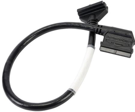
ZIPLink PLC I/O cable, 40-pin connector to 40-pin connector, shielded, 1.6ft/0.5m cable length. For use with BRX series high-speed modules.
