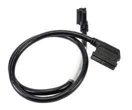
ZIPLink PLC I/O cable, 40-pin connector to 40-pin connector, shielded, 3.2ft/1m cable length. For use with BRX series high-speed modules.
