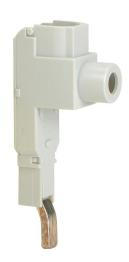
Eaton box type wiring lug, 80A, 480 VAC, 1 openings, #14-2 AWG copper only. For use with ZSVUL series busbars.
