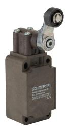
Schmersal IEC limit switch, side rotary lever with plastic roller, 90-degree adjustable head, (2) N.C. contact(s), snap action, 30mm hole spacing, glass-fiber thermoplastic, (1) M20 x 1.5 entry with 1/2in NPT adapter.
