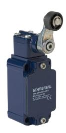
Schmersal IEC limit switch, side rotary lever with plastic roller, 90-degree adjustable head, (2) N.C. contact(s), snap action, 30mm hole spacing, aluminum, M20 x 1.5 entry with 1/2in NPT adapter.
