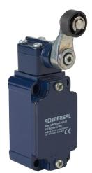
Schmersal IEC limit switch, side rotary lever with plastic roller, 90-degree adjustable head, (2) N.C. contact(s), snap action, 30mm hole spacing, aluminum, (1) M20 x 1.5 entry with 1/2in NPT adapter.
