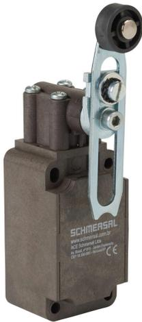
Schmersal IEC limit switch, side rotary adjustable lever with plastic roller, 90-degree adjustable head, (2) N.C. contact(s), snap action, 30mm hole spacing, glass-fiber thermoplastic, (1) M20 x 1.5 entry with 1/2in NPT adapter.
