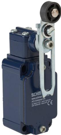
Schmersal IEC limit switch, side rotary adjustable lever with plastic roller, 90-degree adjustable head, (1) N.O./ (1) N.C. contact(s), snap action, 30mm hole spacing, aluminum, (1) M20 x 1.5 entry with 1/2in NPT adapter.
