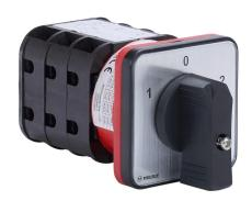
Merz rotary transfer cam switch, 3-pole, 600 VAC, 32A, 5kA SCCR, door mount, front operated. Hardware for 4-hole door mounting & black operating handle included.
