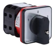
Merz rotary transfer cam switch, 2-pole, 600 VAC, 32A, 5kA SCCR, door mount, front operated. Hardware for 4-hole door mounting & black operating handle included.
